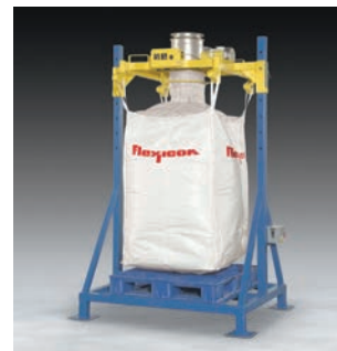
BASIC FILLER for lighter-duty minimizes cost, yet offers an inflatable bag spout seal and feed chute dust vent port, plus optional performance features.
