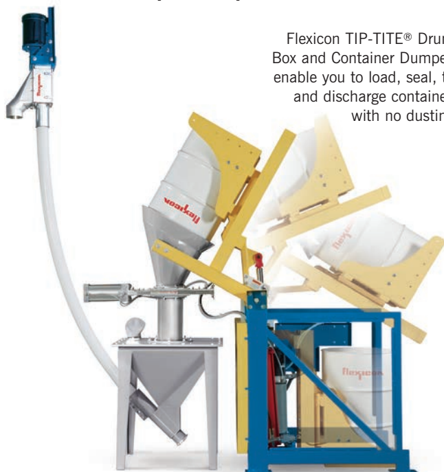
TIP-TITE® Universal Drum Dumper handles drums from 30 to 55 gal (114 to 208 liter). Shown with optional hopper configured with Flexicon flexible screw conveyor. Also available with hopper configured with tubular cable conveyor adapter, pneumatic pick-up adapter, or universal flanged outlet.
