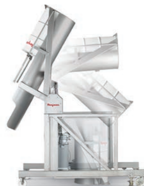
Open Chute Drum Dumper offers a low cost method of discharging free- and non-free-flowing bulk solids when dust generation is not a concern. Discharges directly into process equipment or optional hoppers equipped with conveyor adapters or universal flanges.
