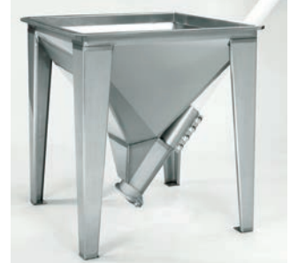
Divergent angles of Flexicon's high flow hopper design reduce the ability of non-free-flowing materials to establish a bridge between the hopper sidewalls, instead causing material to topple and flow toward and down the steep backwall, increasing the flow of bulk materials while decreasing residual material in the hopper.
