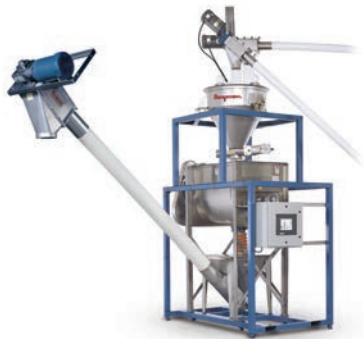
Flexible Screw Conveyors for Weigh Batching/Blending
