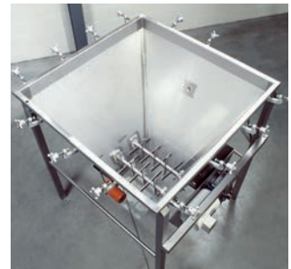
Flexicon offers a multitude of mechanical and pneumatic hopper accessories to promote the flow of poor-flowing or non-free-flowing materials. This hopper features dual agitators with interlocking paddles that de-agglomerate bulk material, promoting void-free charging of mechanical conveyor intake adapters.
