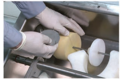
Sanitary Tubular Cable Conveyor Prevents Product, Plant Contamination
