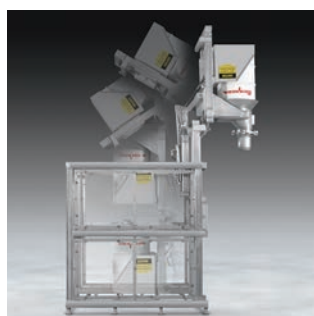
Sanitary TIP-TITE® Drum Dumpers allow loading, sealing, tipping and discharging of drums with no dusting by forming a dust-tight seal between a drum discharge cone and a gasketed receiving ring fitted to existing process equipment or the lid of a hopper.
