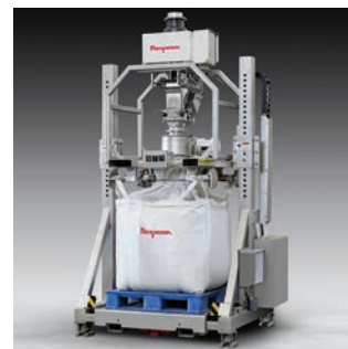
Sanitary TWIN-CENTERPOST™ Bulk Bag Fillers are the first fillers to receive USDA acceptance. They provide a dust-tight, inflatable bag spout seal, a feed chute air-displacement port for dust-free filling, and four-sided access for easy operation and rapid wash down.
