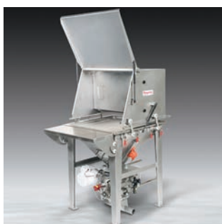
Sanitary Bag Dump Stations with optional dust hoods on rocker arms raise the hood for easy separation and wash down of the gasketed seam—and for removal and wash down of the interchangeable dump screens. Dust collection prevents contamination of personnel and plant environment.
