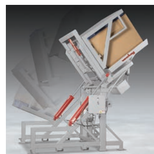
Sanitary TIP-TITE® Box/Container Dumpers form a dust-tight seal between the container rim and gasketed discharge chute. Finished to food and pharma standards, these units provide unrestricted access for rapid, thorough wash down.
