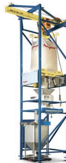
Flexicon's Bulk-Bag-to-Rigid-Bin Weigh Batching System seals against the clean side of the bag spout, elongates the bag for total evacuation, and allows dust-free retying of partially empty bags. A low-profile de-lumping device breaks up agglomerates as a gravimetric feeder loads accurately weighed batches into rigid bins.
