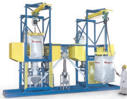
Weigh Batching System with Bulk Bag Dischargers, Educator
