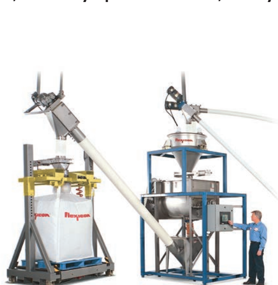
Flexicon's Self-Contained, Gain-in-Weight Batching and Blending System conveys bulk ingredients from multiple upstream sources, weigh-batches, blends and discharges the material into a surge hopper, and transports it to a TWIN-CENTERPOST™ Bulk Bag Filler. The system is offered with Flexicon Flexible Screw Conveyors (shown), FLEXI-DISC® tubular cable conveyors or PNEUMATI-CON® Pneumatic Conveying Systems.
